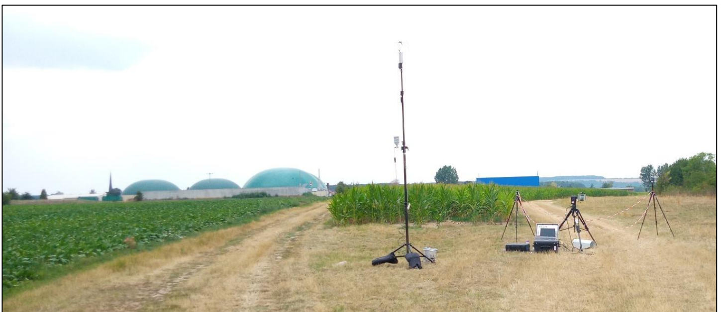
Figure 3: Determination of the total methane emissions with remote sensing from the
