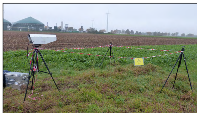
Figure 2: Determination of the overall methane emission rate by means of the Inverse Dispersion Modelling Method. The open-path laser spectrometer measures the atmospheric methane concentration downwind of the investigated biogas plant.
