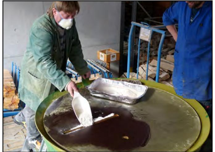
Figure 1. Dosing of kaolin-additive into a mixer with milled fuel prior to palletisation.
