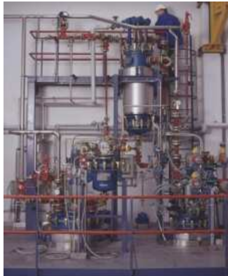
Pilot scale- reactor used for extraction studies
